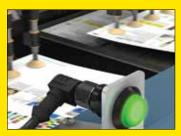
**Collating Machine** S18L and S22L indicators work well for stand-alone use on machines, such as a collating machine to indicate full or empty bins.
