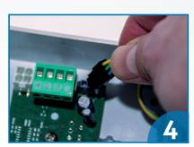
Exchange the sensor cartridge (3) and conncect the cable of the new sensor head to the PCB (4).
